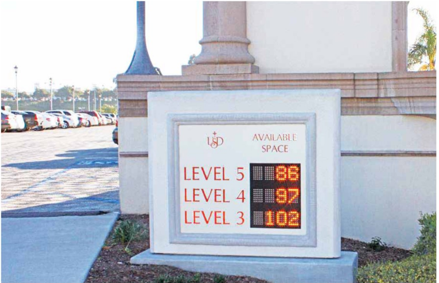
Dynamic signage at parking garages helps prevent motorists from circling completely filled levels.
